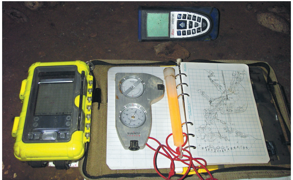
New age surveying tools: PDA with protective case, Suunto Tandem combination compass and clinometer, Leica Disto A6 laser rangefinder, cyalume, and survey notebook. Note the survey book and PDA are mounted on a custom made clipboard for easy transportation underground. Photo by K. M. Kissell
